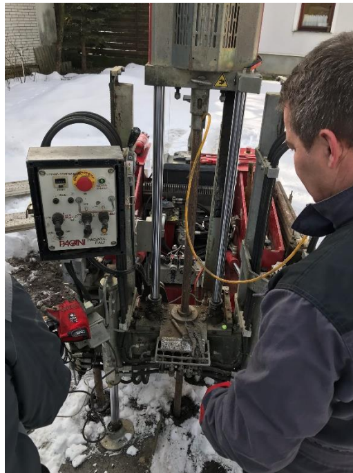
Slika 8: Potiskanje sonde v tla (Vir: https://www.mphisa.si/uploads/1260/img-0019_medium.jpg ( 29.3.2021 ))
