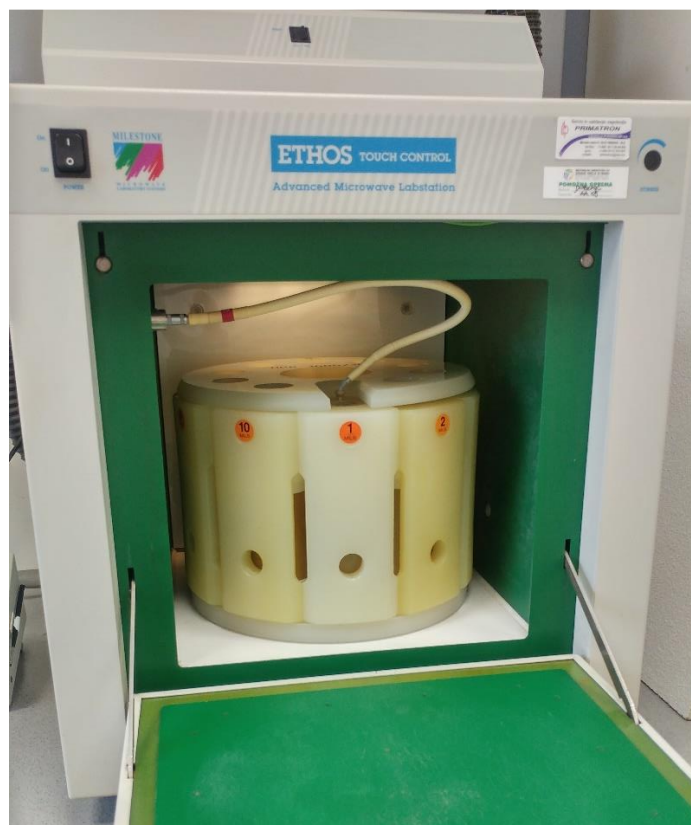
Slika 7 Advanced Microwave Labstation (ETHOS Touch Control) (lasten vir)
