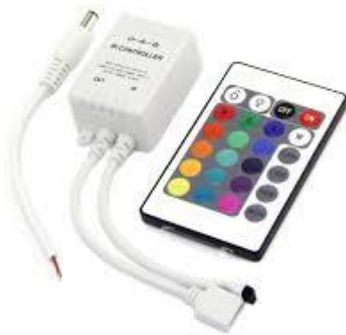
Slika 13: RGB LED krmilnik (vir: https://www.seeedstudio.com/RGB-Controller-p-1093.html )
