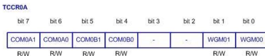
Slika 7: Register TCCR0A (Timer/Counter Control register).
