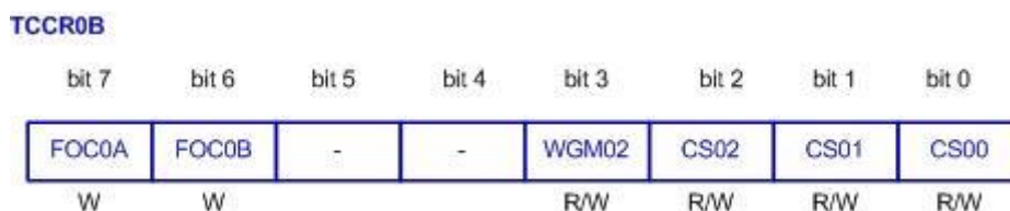
Slika 6: Register TCCR0B (Timer/Counter Control register).
